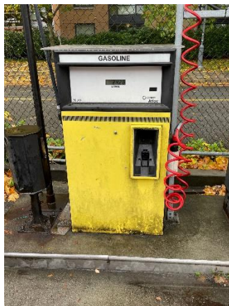
Fig. 2. Fuel pump in on position, scanner (right red cable), nozzle (black left).
